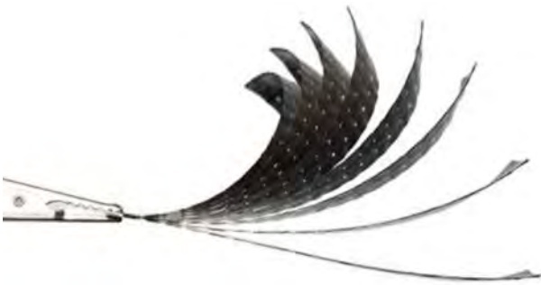
Figure 7. Programmable Adaptable Carbon Fiber (laboratory test coupon).
