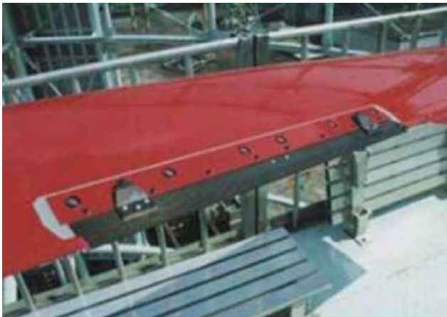
Figure 3. Full-scale rotor blade active flap test
