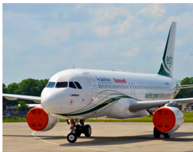
Figure 2. An aircraft with an e-taxi system installed taxiing using only the power from the APU.
