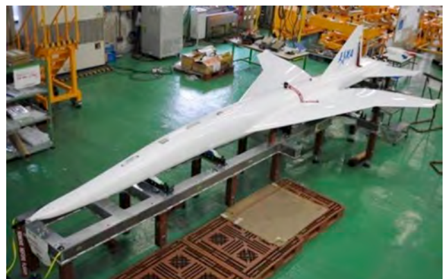
Figure 2. JAXA's Scaled Airplane – Used During Drop Test
