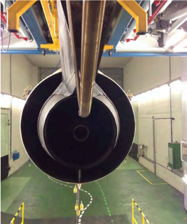
Figure 2. Turboman Engine Seen From Behind With Tube of a Sampling Probe.
