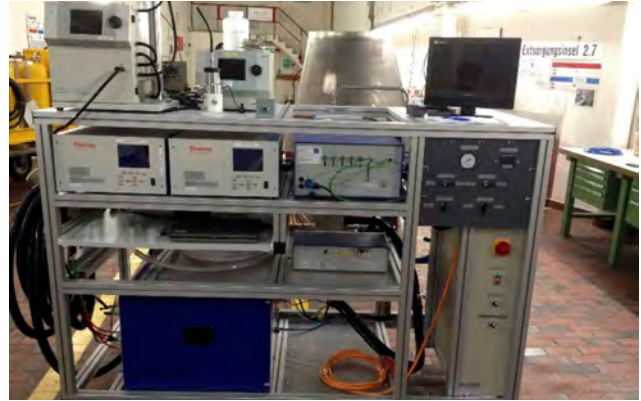
Figure 3. Sections of the Swiss nvPM Sampling and Measurement System With Added Particle Sizing Instrumentation. (Sections 4 and 5 in Figure 4).
