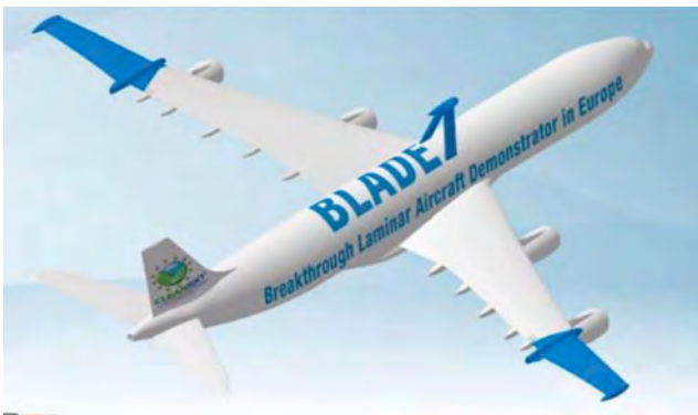
Figure 2. Integrated NLF Design Concepts Installed on A340 Wing Tips of Clean Sky 2 Flight Demonstrator 2 .
